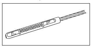
If the oil is below the cross-hatched area (L), you will need to add at least one quart/liter of oil. But you must use the right kind. This section explains what kind of oil to use. For engine oil crankcase capacity, see *Capacities and Specifications on page 5-100*.
